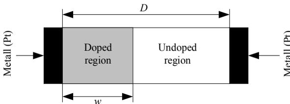
Fig. 1.19. A simple physical model of the memristor
