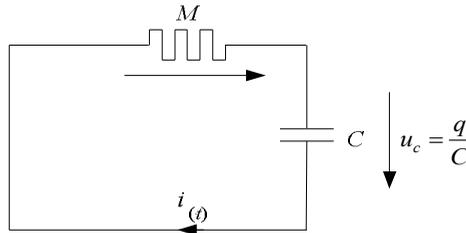
Fig. 4.5. The circuit of discharge of the capacitor
