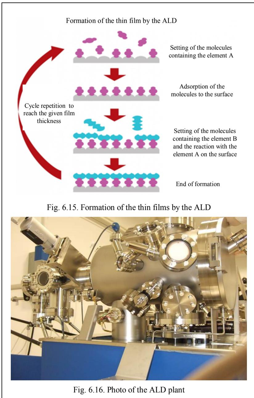
To form the functional layer of the dielectric in the MDM (MIM) structure the atomic-layer deposition method is used because it has unique ability to obtain the homogeneous thin films of a given thickness (a few nanometers) and to control their composition. As already noted, the oxygen vacancies play a key role in the effect of the resistive switching.
