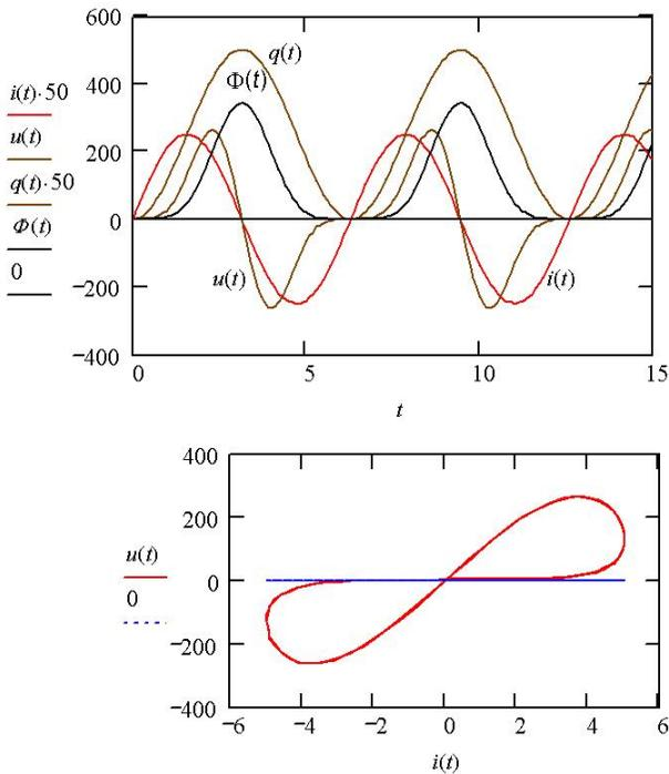
Fig. 1.11. The response of the memristor on the amplitude of action equaled  $I_m = 5 \text{ A}$
