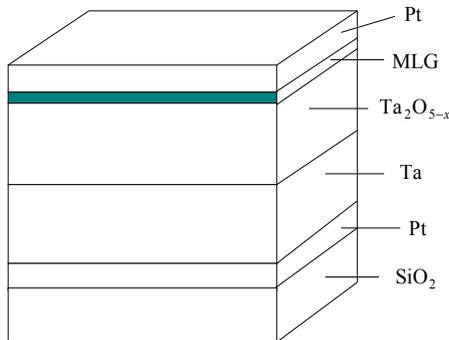
Fig. 7.5. Memory cell structure of the ReRAM type
