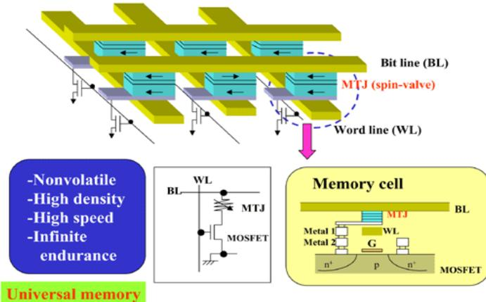
Fig. 7.17. The technology of manufacturing the memory matrix
