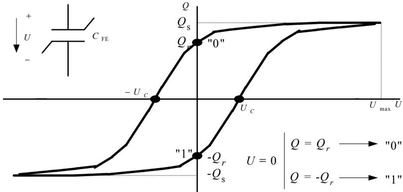
Fig. 7.30. The hysteresis loop of the ferroelectric capacitor
