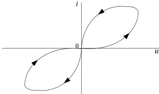
Fig. 1.22. The dependency  $i(u)$  of the memristor
