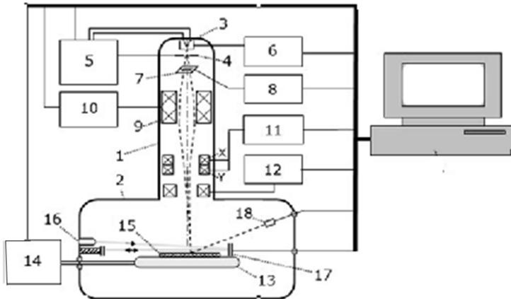
Fig. 6. 5. Block diagram of the electronic lithography system
