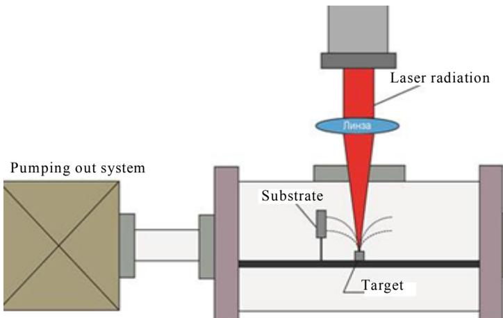
Fig. 6.17. Laser ablation of the target material
