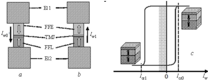
Fig. 7.54. The structural diagram of the memory cell
