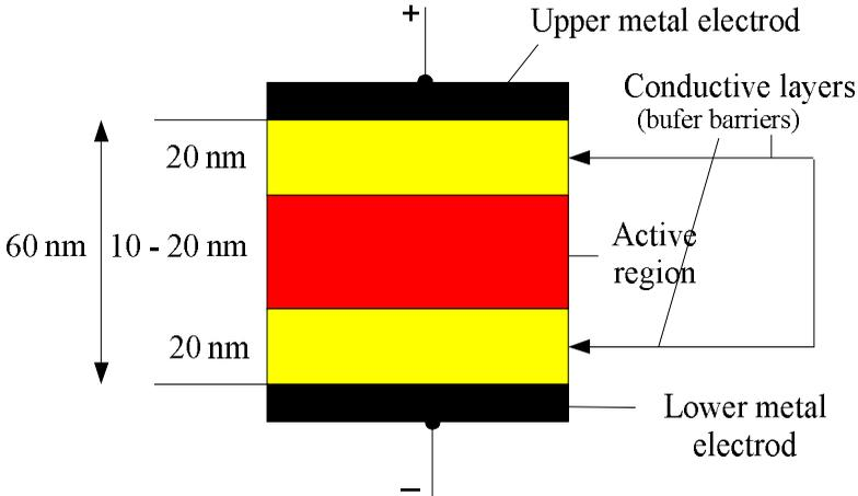
Fig. 7.37 The structure of the CeRAM memory cell
