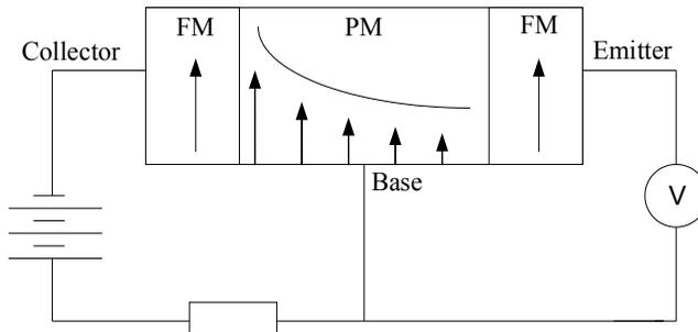
Fig. 7.11. The structure of the Jonson transistor
