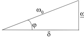
Fig. 4.11. The relationships between the frequencies in *RLC*-circuit
