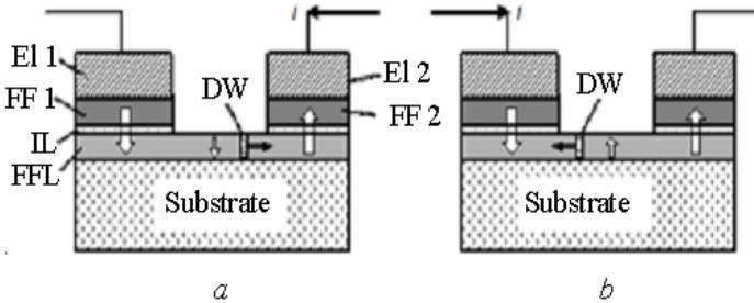
Fig. 7.43. Process of the spin-transport magnetization reversal
