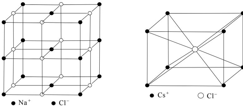
Fig. 7.26. The elementary cells of the lattices
