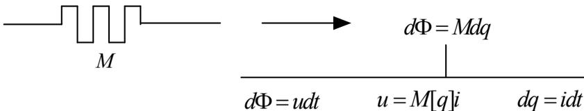
Generally memristance  $M$  should depend on the charge  $q$ . If a magnetic flux is represented by the time integral of the voltage then using the relations  $d\Phi = udt$  and  $dq = idt$  it is possible to write the relationship between current and voltage in the form:
