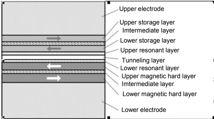
Fig. 7.20. Multilayer architecture of the MRAM cell
