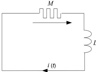
Fig.4.8. Electric  $ML$  – circuit with the initial current
