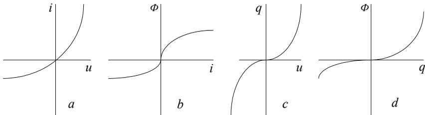
Fig. 1.15. Characteristics of the four fundamental elements
