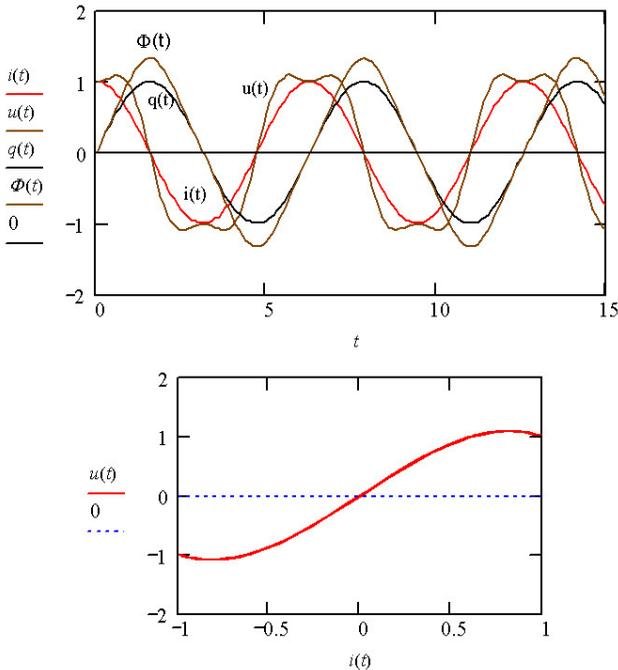
Fig. 1.13. Hysteresis loop degenerates into single-valued function
