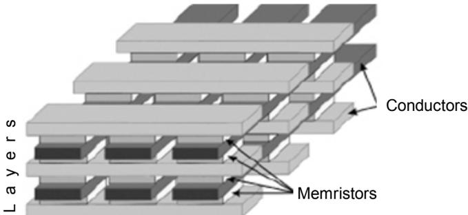
Fig.7.2. Forming 3D structure of the ReRAM memory
