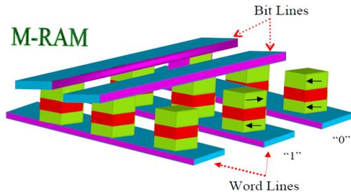
Magnetic tunnel junction is used to create the magnetic random access memory. The value of the MTJ transition resistance determines whether the resistance of the cell will read as "0" or "1", when the read current passes through the cell.
