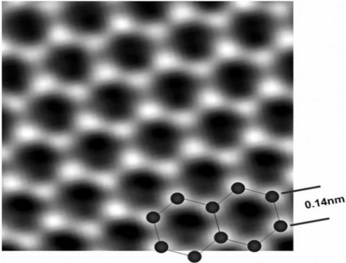
Fig. 7.6. Image of the graphene structure obtained by the atomic force microscope
