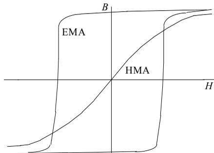
When the film thickness decreases to a few hundred Angstroms the magnetic film becomes the single-domain magnetic film with respect to its thickness. In this case a little time switching films ( $\sim 10^{-9}$  s) and high operation speed of the magnetic elements may be provided.
