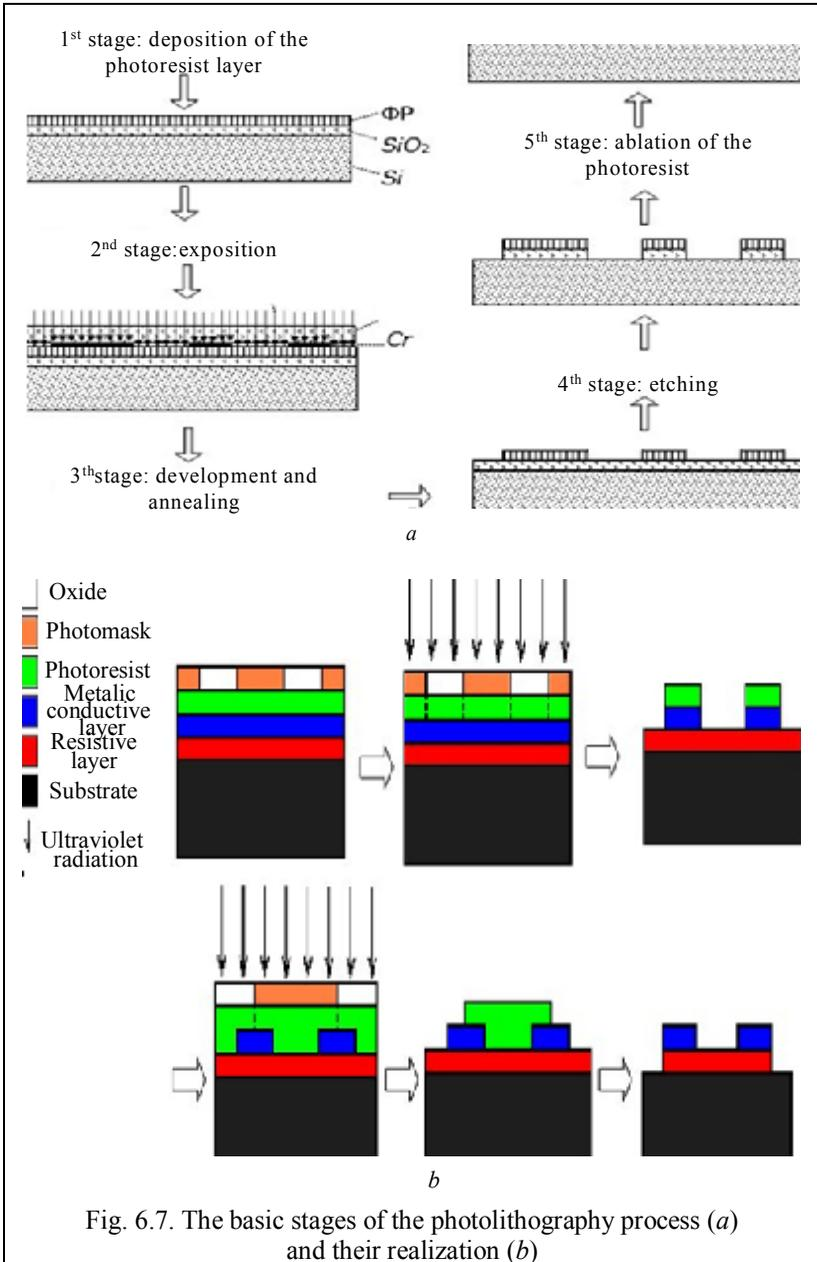
Fig. 6.7. The basic stages of the photolithography process (a) and their realization (b)
