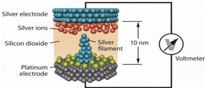
Fig. 5.13. Formation of the filament in the structure Ag/SiO<sub>2</sub>/Pt
