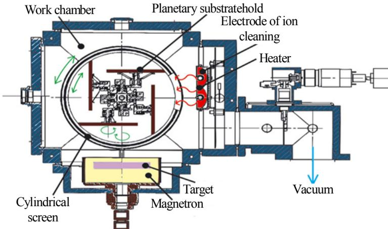
Fig. 6.13. Block diagram of the magnetron deposition plant
